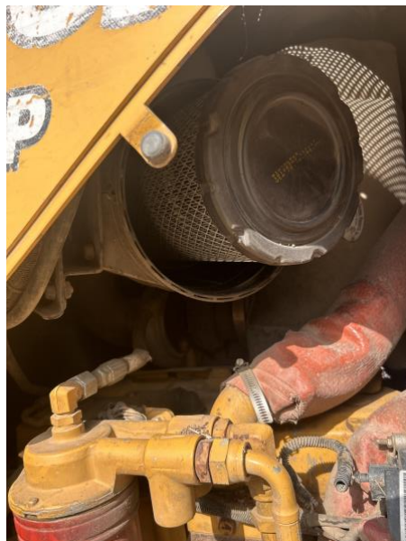
Photo 6: Outer Air Filter
