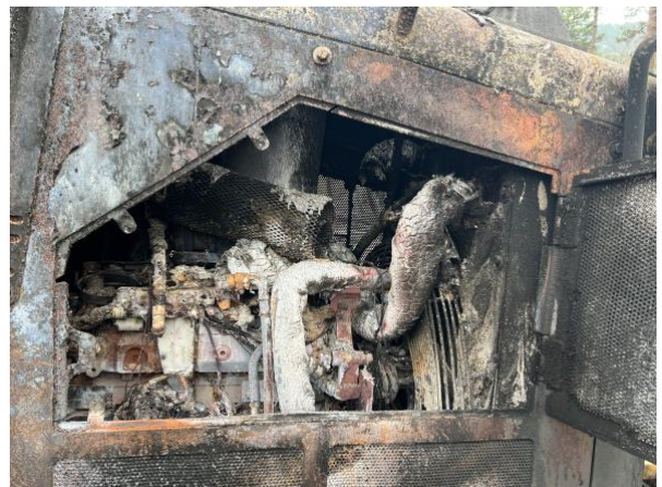
Photo 4: Access Point to Air Filter Housing
